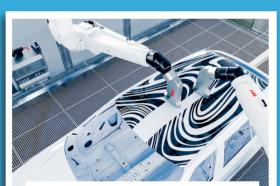
ABB's painting robots use a special printer head to enable mass customization vehicle finishes at half the usual cycle time.
