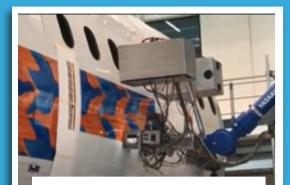
Dutch robot manufacturer XYREC uses inkjet technology to print a large image on an Airbus A320 fuselage.
