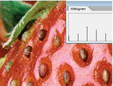
A typical ScreenPro output image with 5 printable levels (4 drop sizes) available for each individual pixel - the histogram shows the distribution of the individual pixels across the 5 levels available.
